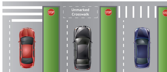
Examples of a few of the most common types of crosswalk markings. Please, be aware that there are other types as well.
